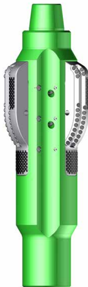
12 ¼" Pilot PDC Hole Opener fitted with 17 ½" reaming blades
